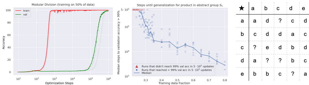
Figure 1: Left. Grokking: A dramatic example of generalization far after overfitting on an algorithmic dataset. We train on the binary operation of division mod 97 with 50% of the data in the training set. Each of the 97 residues is presented to the network as a separate symbol, similar to the representation in the figure to the right. The red curves show training accuracy and the green ones show validation accuracy. Training accuracy becomes close to perfect at < 10^3 optimization steps, but it takes close to 10^6 steps for validation accuracy to reach that level, and we see very little evidence of any generalization until 10^5 steps. Center. Training time required to reach 99% validation accuracy increases rapidly as the training data fraction decreases. Right. An example of a small binary operation table. We invite the reader to make their guesses as to which elements are missing.
