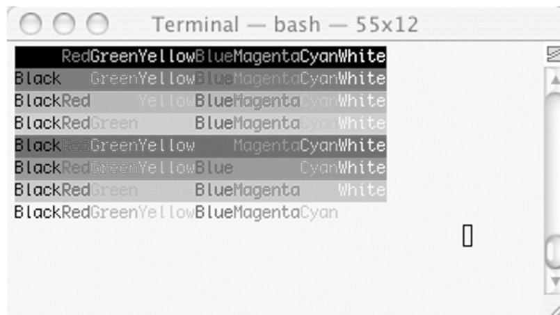
Figure 6-2. The text and background colours can be changed.
