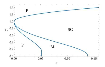
Figure 1. Phase diagram of the Hopfield network. The phase diagram lives in the  $(\alpha, \beta)$  plane. In the upper region (P) the network behaves randomly while in the top-right region (SG) it is frozen in a spin-glass phase. The working regions are solely the two down-left where patterns are global minima of the free energy (F) or relative minima of the free energy (M).
