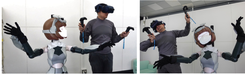
Figure 5: Hatsuki can be teleoperated. Our system uses the operators head and body postures, facial expressions, and voice to control Hatsuki and deliver interactive anime-like performances.
