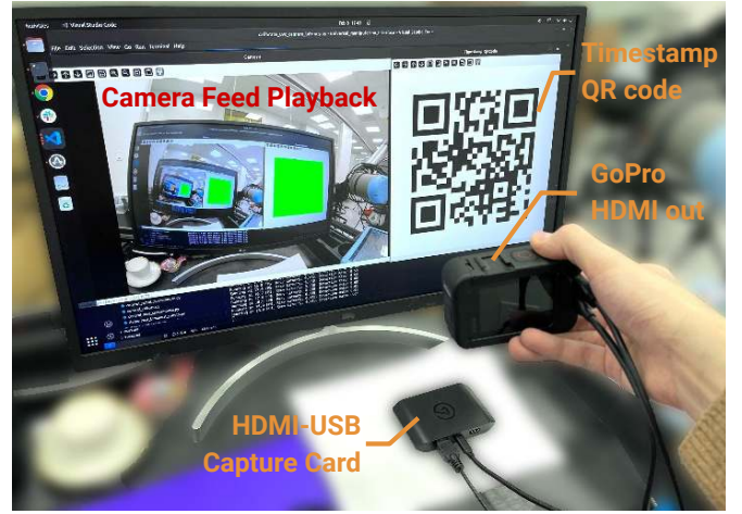
Fig. A1: Camera Latency Measurement
