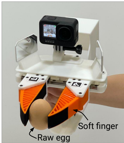
Fig. A3: Soft Fingers printed with TPU material provides passive mechanical compliance, enabling a secure grip on a raw egg without causing breakage.
