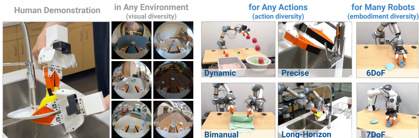
Fig. 1: Universal Manipulation Interface (UMI) is a portable, intuitive, low-cost data collection and policy learning framework. This framework allows us to transfer diverse human demonstrations to effective visuomotor policies. We showcase the framework for tasks that would be difficult with traditional teleoperation, such as dynamic, precise, bimanual and long-horizon tasks.
