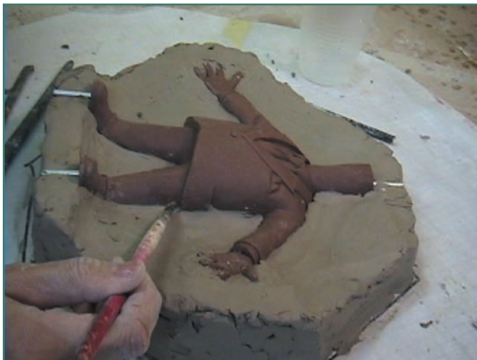
Figure 7.53 Building up a clay bed around the sculpt. (Copyright Zung Studio.)
