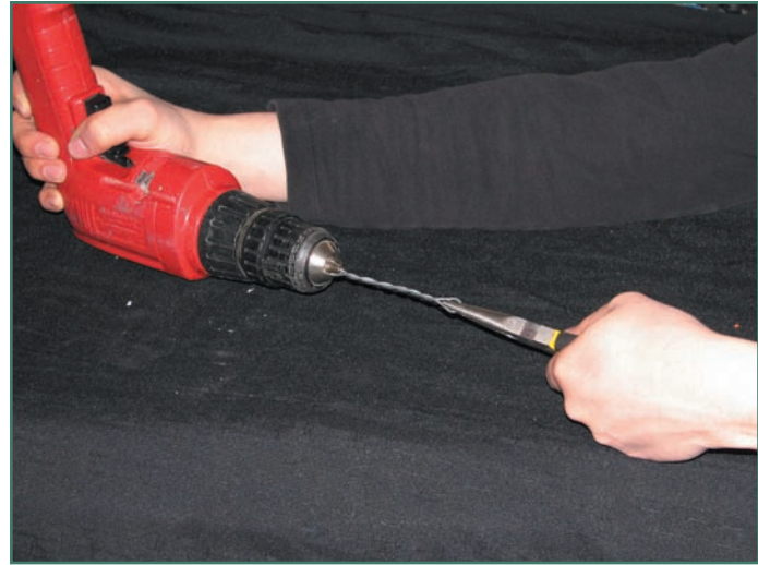
Figure 7.32 Twist the wire with a power drill.
