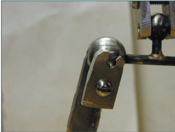
Figure 7.29 Hip joint designed by Tom Perzanowski, with a notch in the socket for greater freedom of movement. (Courtesy of Larry Larson at Center for Creative Studies.)
