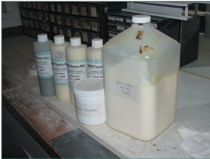
Figure 7.58 A foam latex kit: base with foaming, curing, and gelling agents. (Courtesy of the Clayman's 3D Cartoon Communications.)
