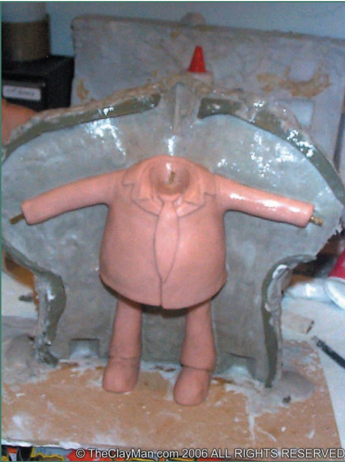
Figure 7.55 The first half of the mold with the sculpt embedded inside. (Courtesy of The Clayman's 3D Cartoon Communications.)
