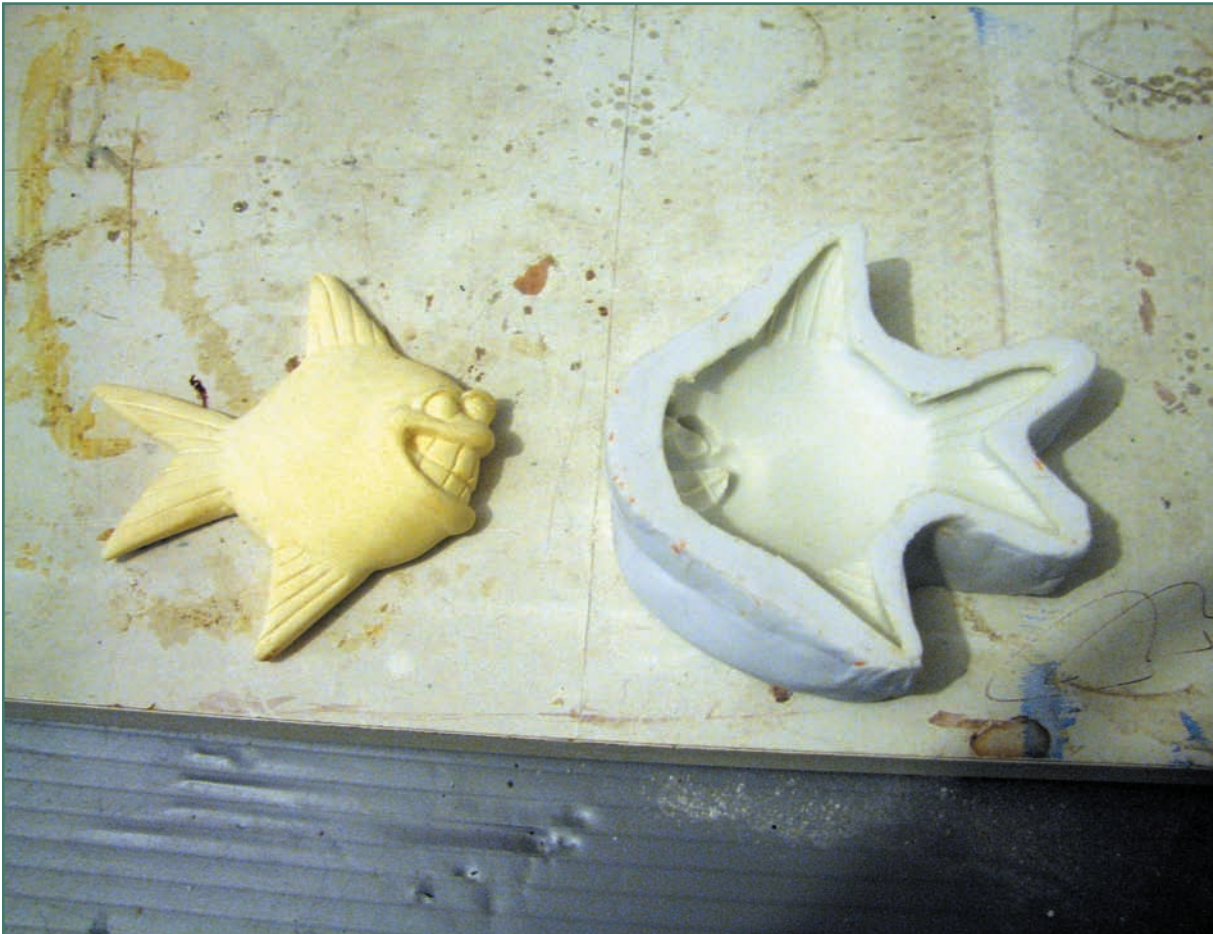
Figure 7.65 Soft rubber mold with poly resin sculpture. (Courtesy of the Clayman's 3D Cartoon Communications.)
