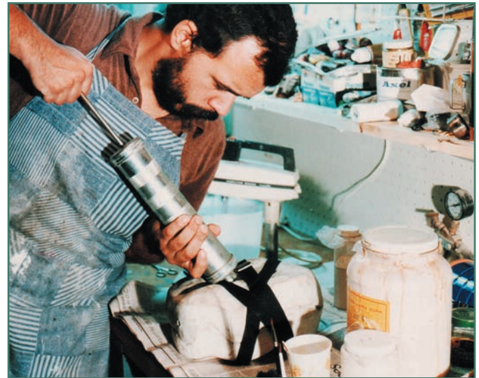
Figure 7.59 Injecting foam latex into the mold. (Copyright Stop Motion Works.)
