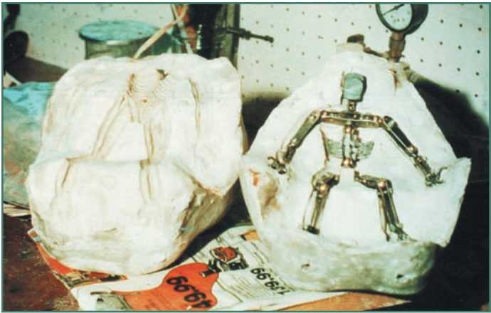
Figure 7.57 Both halves of the open mold, with armature laid inside. (Copyright Stop Motion Works.)
