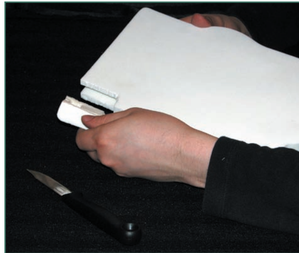
Figure 7.34 Feet can be made from pieces of foam.
