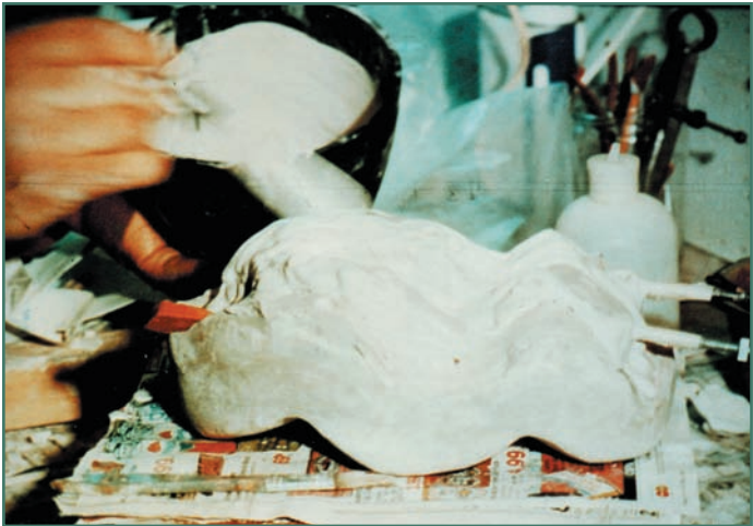
Figure 7.56 Applying a gypsum material to the mold to create the second half. (Copyright Stop Motion Works.)
