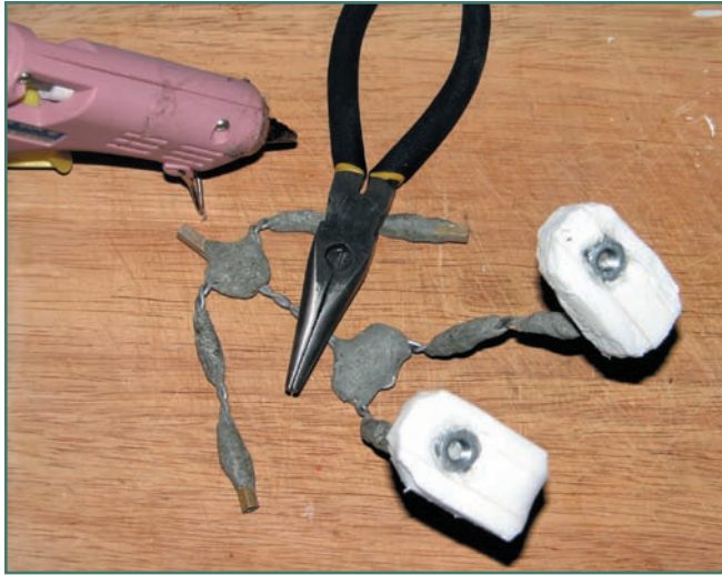
Figure 7.40 Tie-downs are glued into the bottom of the feet.
