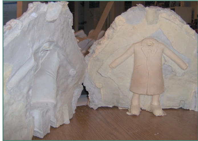
Figure 7.60 The mold is pried open to reveal the latex puppet inside. (Courtesy of the Clayman's 3D Cartoon Communications.)
