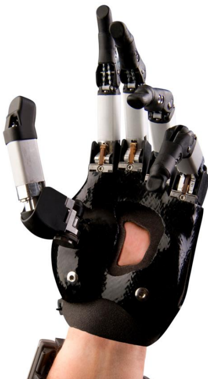
Figure 2.10 – iLimb Digits attached to an amputee four fingers and the thumb but palm still intact (courtesy Touch Bionics)
