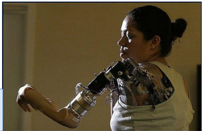
Figure 1.3 – Advanced DARPA myoelectric prosthetic arm
