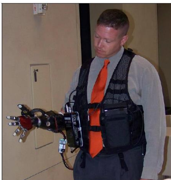
Figure 2.20 – APL intrinsic hand being used by an amputee (courtesy John Hopkins APL)
