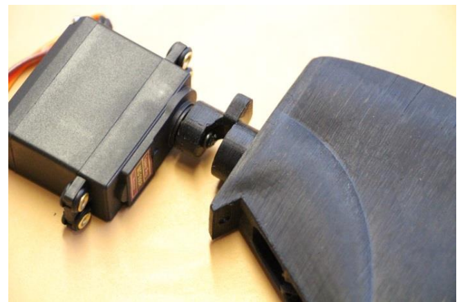
Figure 3.9 – Improved wrist rotation mechanism
