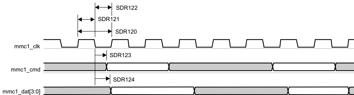
Figure 7-65. MMC/SD/SDIO in - High Speed SDR12 - Transmitter Mode
