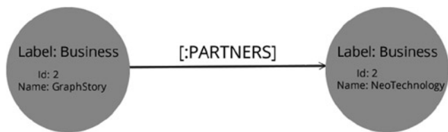
Figure 3-6. Bidirectional relationship with an arbitrary direction
