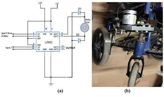
Fig. 3. (a) Circuit diagram of a motor driver L239D IC (b) ASMC-04 digital servo for steering the front wheel.
