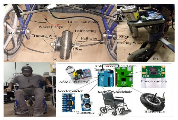
Fig. 4. Wheelchair assembly with components.
