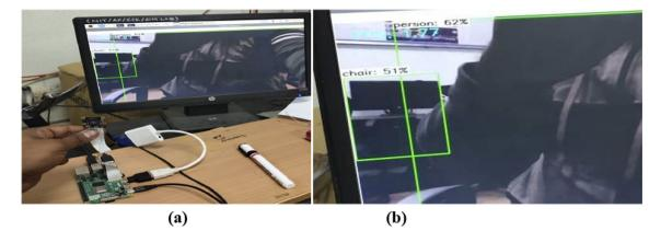
Fig. 5. (a) Pi camera is connected with Raspberry pi (b) System is detecting a chair.
