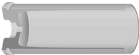
Cross section of a cartridge case, Image courtesy of Federal Cartridge Corp.
