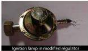
Ignition lamp in modified regulator
