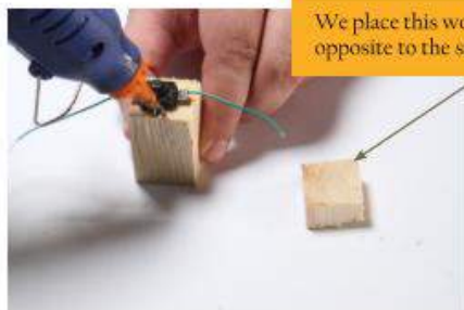
5. Fix the Push-Switch in the wooden piece using glue.
